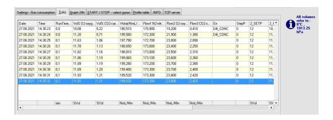
This table shows all data - measured and calculated data during operation.
