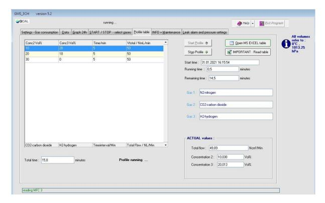
This function allows to run a concentration – time – profile automatically. The gas for each channel is indicated at the footer of the table.
