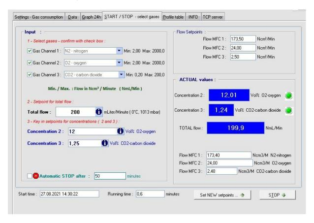
For manual operation mode it is necessary to enter data in the frame *Inputs*:
